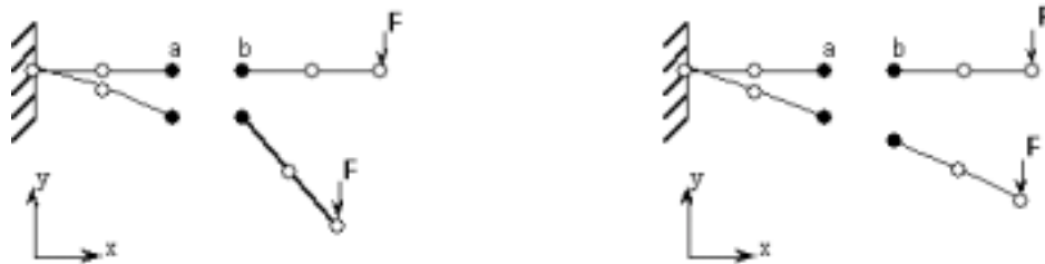
Offset nodes a and b are constrained to move together.
